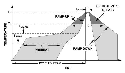
Figure 12 Recommended Soldering Profile
