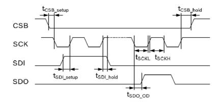
Figure 4 SPI timing diagram
