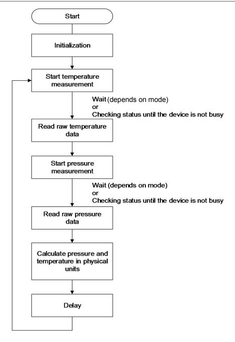
Figure 2 Measurement flow of WF5805F
