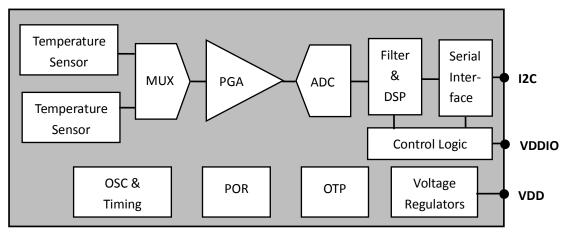
Figure 1 Block diagram of WF5805F
