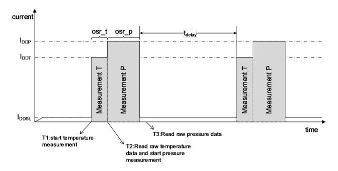
Figure 3 Recommended working timing diagram
