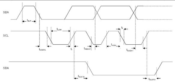
Figure 7 I2C Timing Diagram
